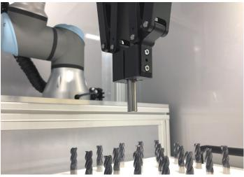
An industrial robot integrated into the **Workstation Robotic** automatically removes objects from a pallet and replaces them afterwards. Six articulated joints allow free movement anywhere within the laser station. This means that there are fewer steps for the user to perform and cycle times are therefore reduced. Especially when handling delicate components, robots offer considerable potential savings through improved product quality.
